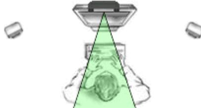
While this document talks about a 30 degree cone, the width of the cone is determined by the spacing between the two microphone elements. The following table shows the cone width at the indicated microphone spacing.
